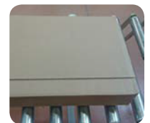
4. Upper flaps sealed with glue.
